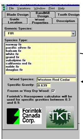
Choose the wood species and specific gravity (density) of the wood you are cutting from a list of common commercial wood species. This information is needed for calculating power requirements and sawing deviation.
